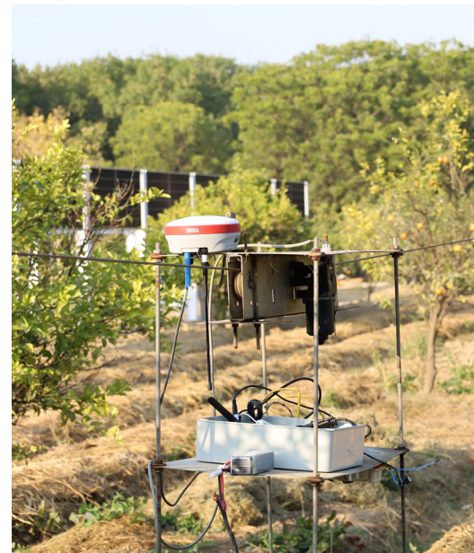
A state-of-the-art trolley robot for the Crop Phenotyping Application at the Digital Agriculture Field at LUMS
